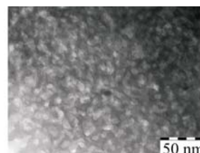
Fig. 15 Pd-doped TiO 2 film obtained from nanopowder (MTP), thermally treated at 500°C
